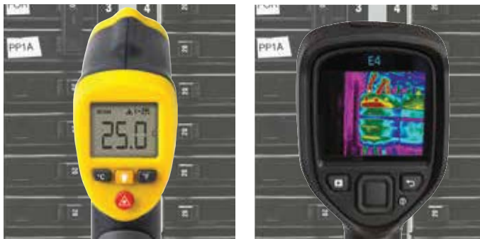
IR thermometer, temperature measurement in one spot FLIR E4, temperature in 4,800 spots
