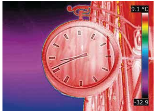
Thermal image with MSX®: Although glass is not transparent for infrared radiation this thermal image clearly shows the hands of the clock behind the glass. This is only possible thanks to MSX® technology that overlays a part of the visual image over the thermal image. The result: thermal images on which the smallest details can be seen.
